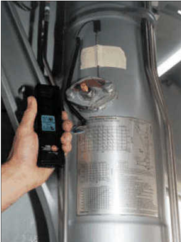
TOP CHARGING VALVE TEMPERATURE MEASUREMENT
