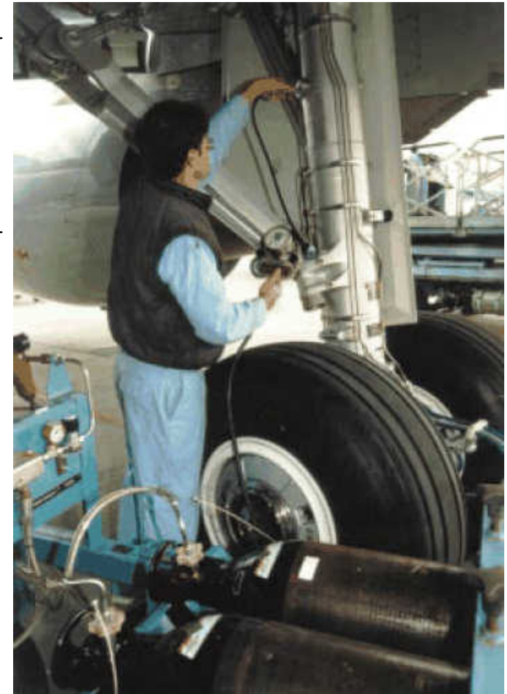
SHOCK ABSORBER NITROGEN SERVICING
